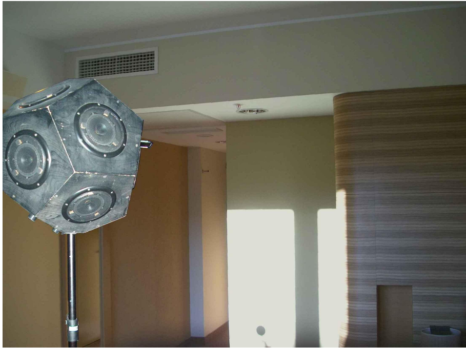
Fig.1. Measurement situation in source (primary) room.
